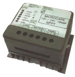
Via links the load voltage disconnect can be selected, whether the battery is lead acid or sealed, and whether the unit operates as a normal load shedder or as a day/night switch.
